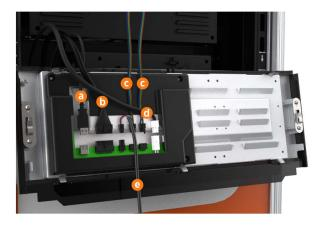
21. Angle the top edge of the LED display under the light bar on the Express 250. Starting at the top, align and slide the LED display guide tabs into the corresponding slots. Ensure the lower sign is correctly captured by the bottom edge of the LED display. Push the bottom into place until firmly seated.
