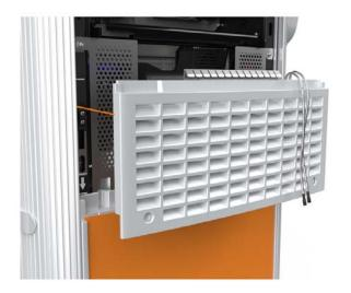
11. You should now be able to remove the orange ChargePoint sign from the lower portion of the unit, and slide the new one into place.
